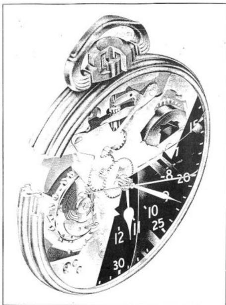
Figure 2—Three-quarter Cutaway View of Hamilton Master Navigation Watch
